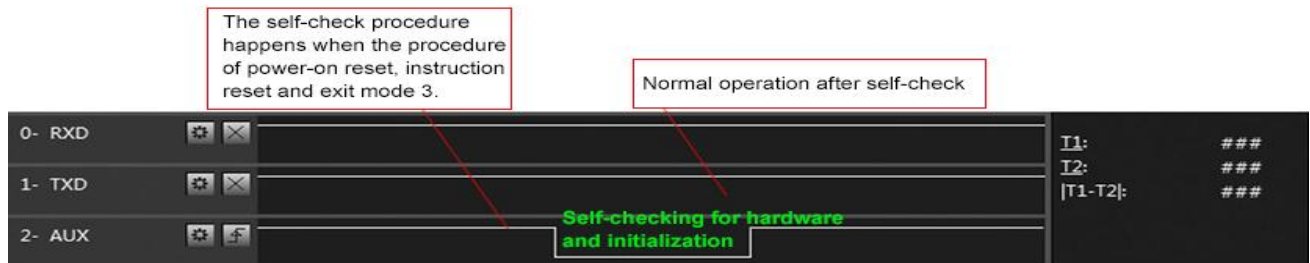
Timing Sequence Diagram of AUX when self-check
