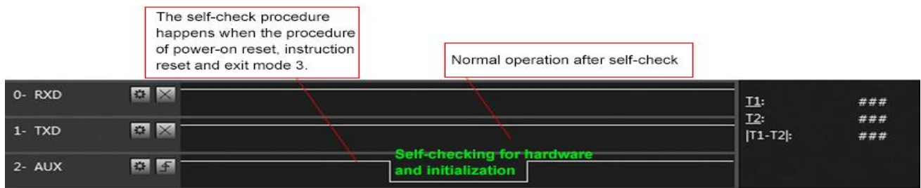
Timing Sequence Diagram of AUX when self-check
