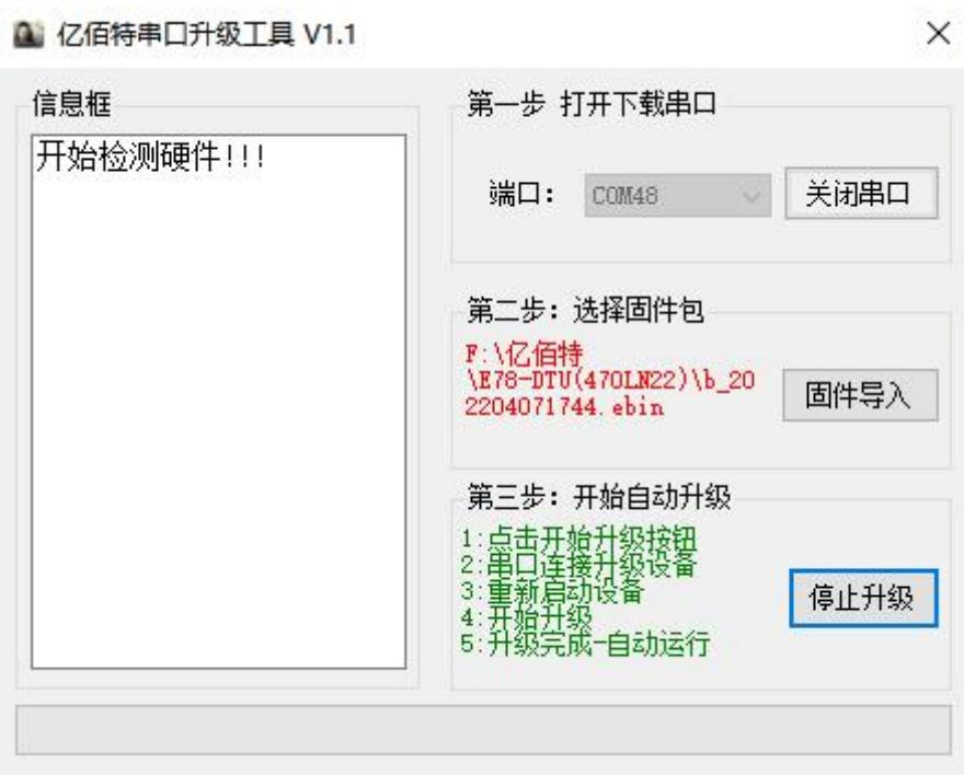
At this time, power on the device that needs to be upgraded, and then it can be upgraded by itself.
