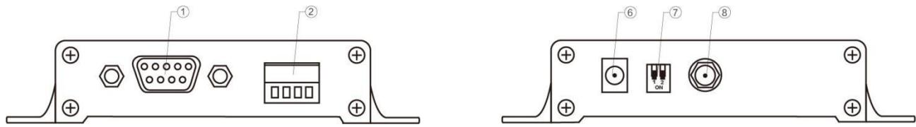
Users can choose ⑥ DC power interface for power supply, and use the interface to supply power to the power adapter with an outer diameter of 5.5mm and an inner diameter of 2.5mm;
