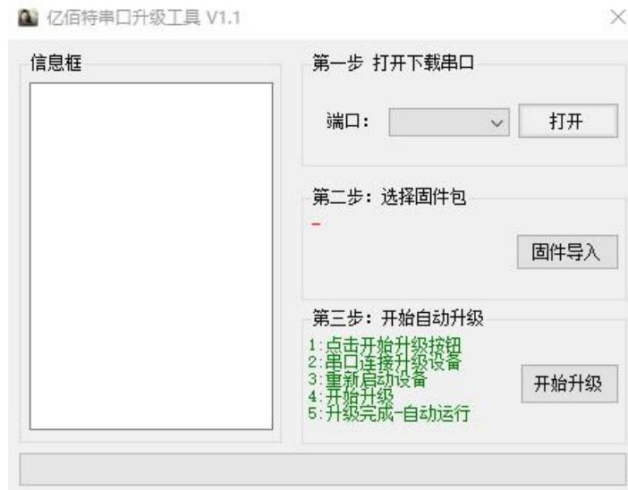
Select the corresponding port and open it, select the firmware package to be upgraded, and click to start the upgrade after importing.
