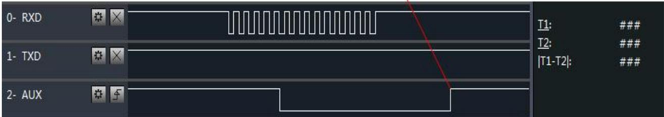
Timing Sequence Diagram of AUX when RXD pin receives
